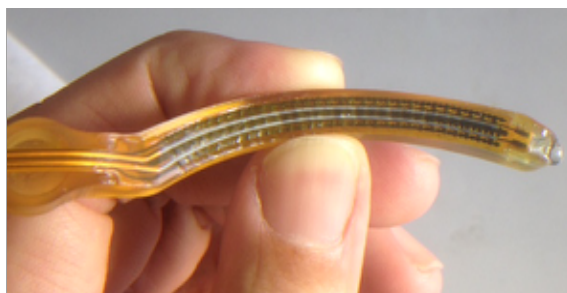
Fully Assembled Lower LClamp Jaw With Sophisticated LED, PTC, and RF on Flex Circuit
